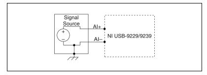
Figure 8. Connecting a Grounded Signal Source to the NI USB-9229/9239
